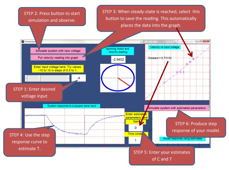
USERS should <u>repeat steps 1 to 3</u> for a wide range of voltages in order to get a large scale view of the velocity dependence upon voltage and whether this is in deed presented by a straight line. [WARNING: when 1<sup>st</sup> opened it can take a while for the 1<sup>st</sup> value to run as MATLAB is opening relevant files/toolboxes so please be patient before moving to the 2<sup>nd</sup> value of voltage].
