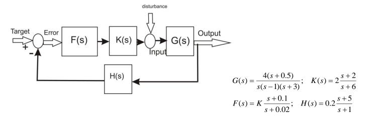
Sketch the root-loci for the following systems. Propose values for compensator gain K.
