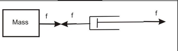
In this arrangement, one end of the damper is fixed and thus does not move. Also, this is NOT a series arrangement even though it may appear so because:
