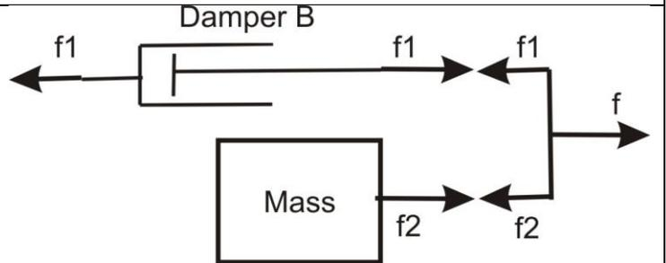
In a series arrangement, the same force that is going through the damper, also applies to the mass, but the extension of the damper and movement of the mass need not match although the movements must match at the point where connected.
